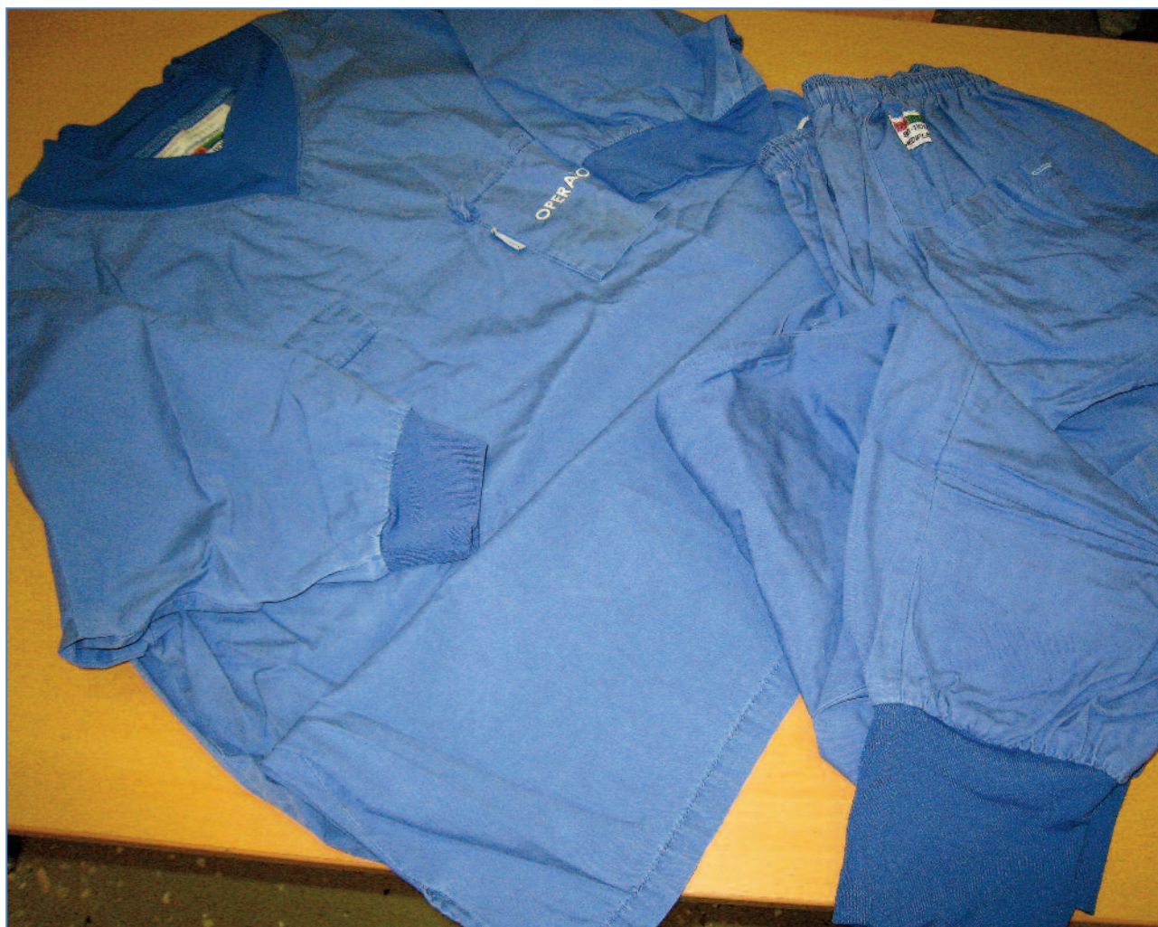
Figure 3. Surgical clothing system of mixed material, 69% cotton, 30% polyester and 1% carbon fibre.
